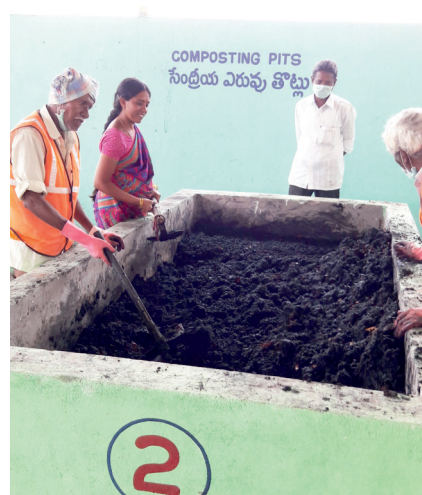
Churning of waste in the pit
